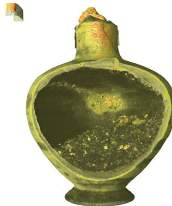
VIRTUAL CUT OBTAINED THROUGH NEUTRON TOMOGRAPHY OF ETRUSCAN VASE ( ARYBALLOS )
