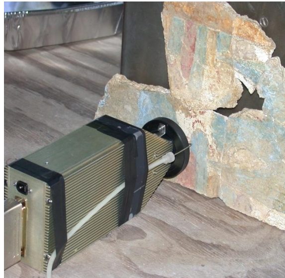
PIXE-ALPHA SPECTROMETER DURING A MEASUREMENT OF A FRESCOES BELONGING TO THE NESTOR PALACE WALL PAINTINGS IN PYLOS (GREECE)
