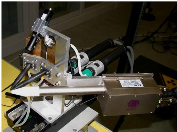
The measurement head of the XRF spectrometer of LABEC
