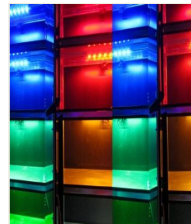
Spectral cabinets developed specifically to test the effect of monochromatic light on phototrophic biofilm growth
